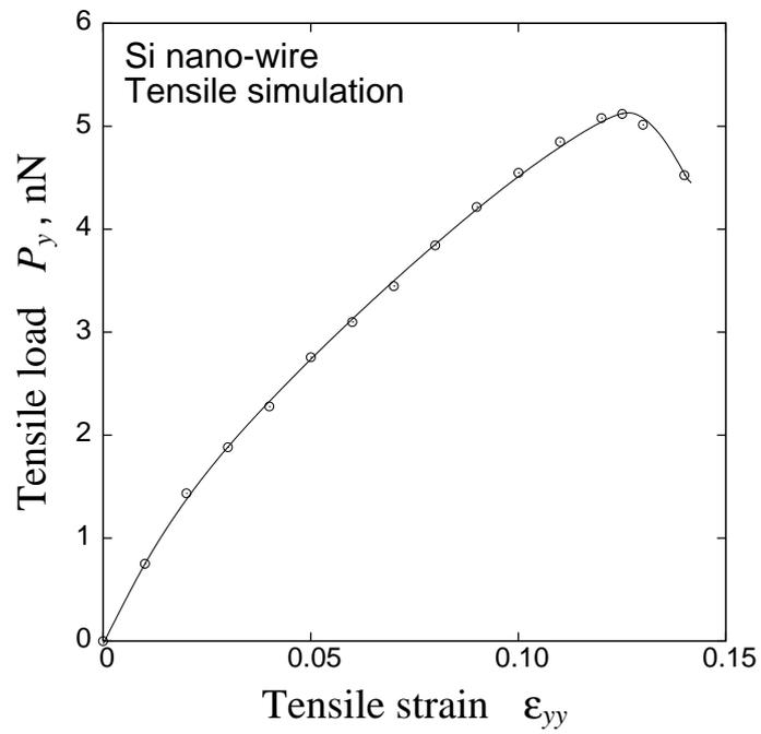
(b) Relationship between the external tensile load and the strain.
