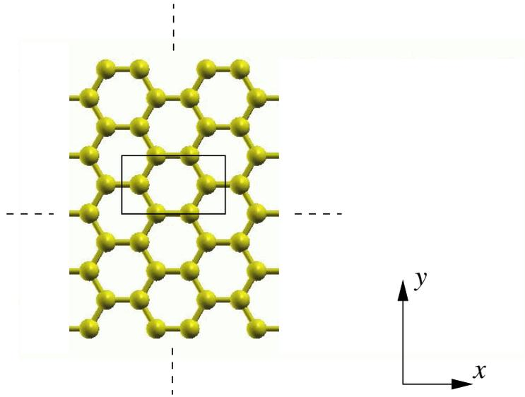
(a) Ideal structure of carbon layer in graphene sheet and the unit cell for calculation.
