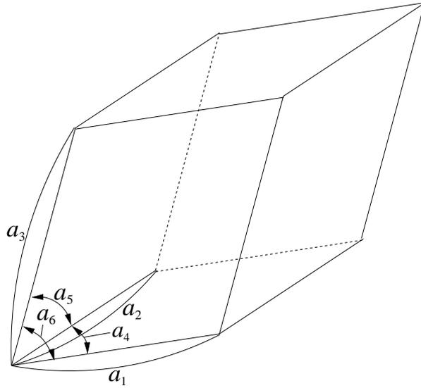
Figure 8: Variables  $a_1 - a_6$  that represent the deformation of unit cell.
