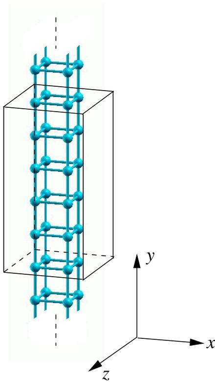
(a) Structure of nano-wire (5 cubes) for analysis of buckling.
