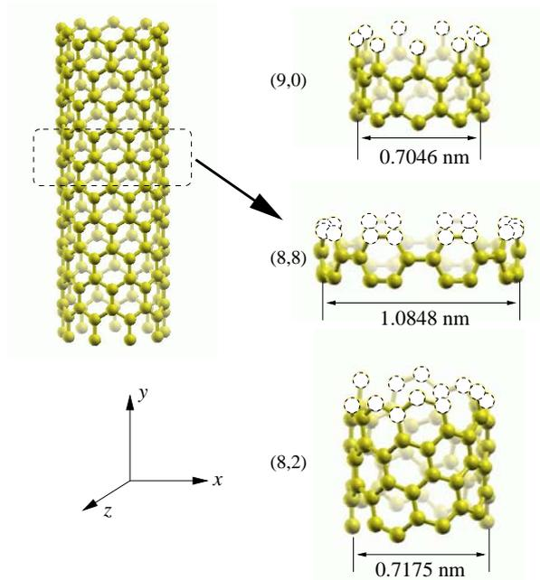
(a) Structure of carbon nano-tubes, (9,0), (8,8), (8,2), and their unit cells.
