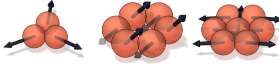
Figure 13: The magnetic ordering for Mn clusters on a Cu(111) surface according to calculations by Bergman et al. [18].
