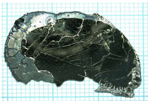
Figure 1: Ba(Fe 0.80 Co 0.20 ) 2 As 2 single crystal: cleavage plane and lobed edges
